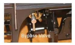
With careful adjustment of this valve, the engine will always have enough water to keep running for long periods of time until the tender water tank needs to be refilled. The tender is also equipped with the hand pump, which needs to be used to prime the axle pump. Only two or three strokes are necessary to prime the pump.
